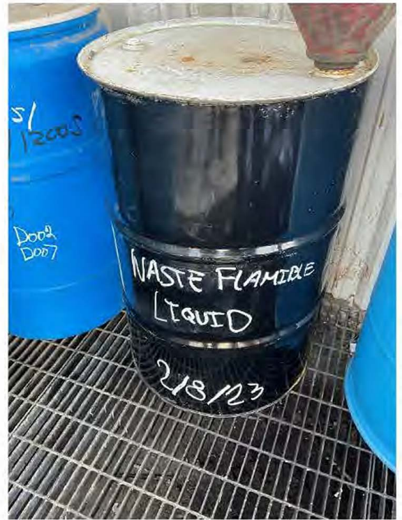
014 March 14, 2023 Williams International Co. A 55-gallon drum not properly marked/labeled with the words "Hazardous Waste."
