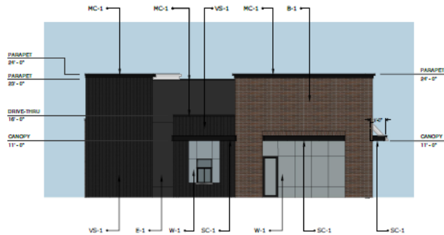
LEFT ELEVATION (WEST) SCALE: 1/8" = 1'-0"
