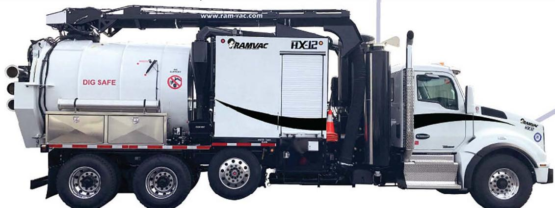
RAMVAC's boom features a 5' extension for a total reach up to 26' from the truck. Worm gear driven, with access to the receiver box, and a abrasion-resistant steel at the back to absorb the impact from bulk material. RAMVAC's standard "dig deep" boom provides operators the ability to dig 13 feet below grade utilizing one standard vacuum tube.
