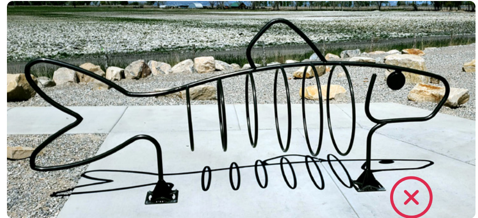
Skipper Bay Trailhead - the June Sucker "ribs" are placed too close together, making it difficult to lock bikes between them. Consider spacing them at least 2 feet apart.
