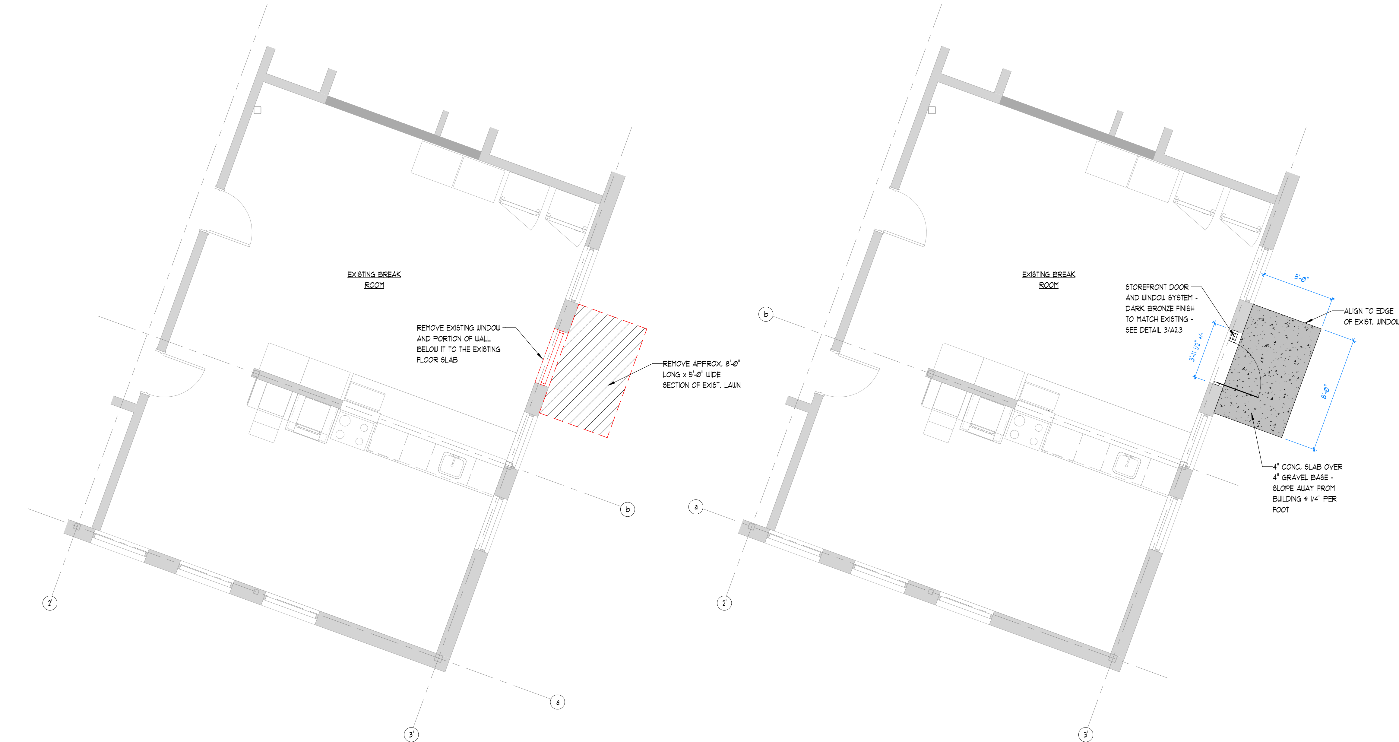
1 ENLARGED BREAK ROOM DEMO PLAN 1/4" = 1'-0"
