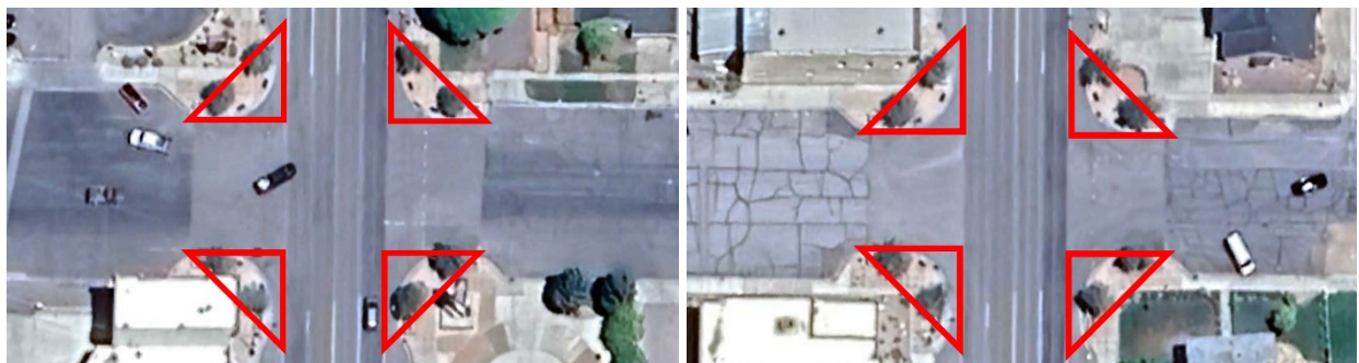
Figure 3: Red triangles outline the clear view area required by Section 1624 Gunnison Land Use Ordinance. Planter boxes and trees are within the required clear view area. Main Street and Center Street (Left). Main Street and 100 South (Right).
