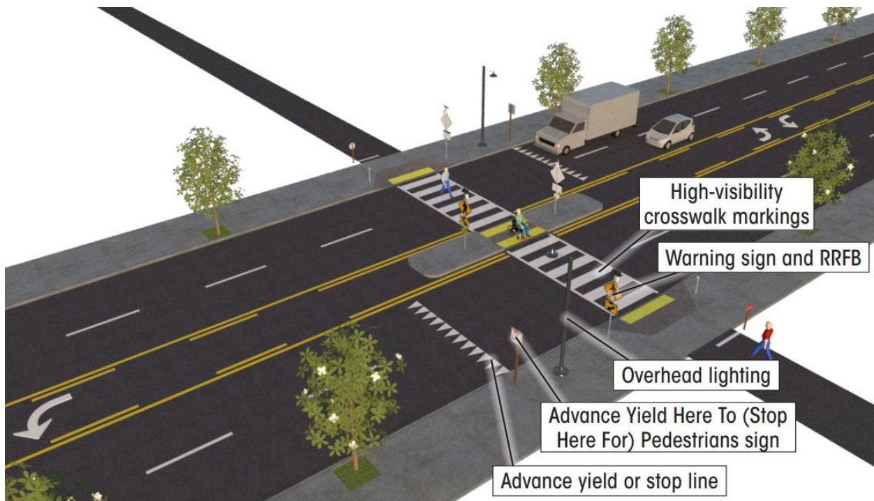
Figure 2: Function of a rectangular rapid flashing beacon and crosswalk.
