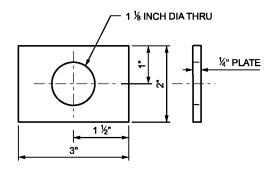
**PLATE WASHER** (2 REQUIRED EACH BOLT)
