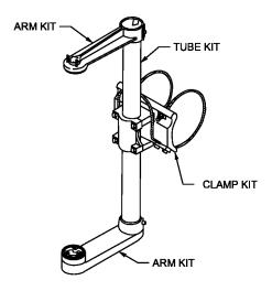
SIGNAL HEAD MOUNTING BRACKET DETAIL
