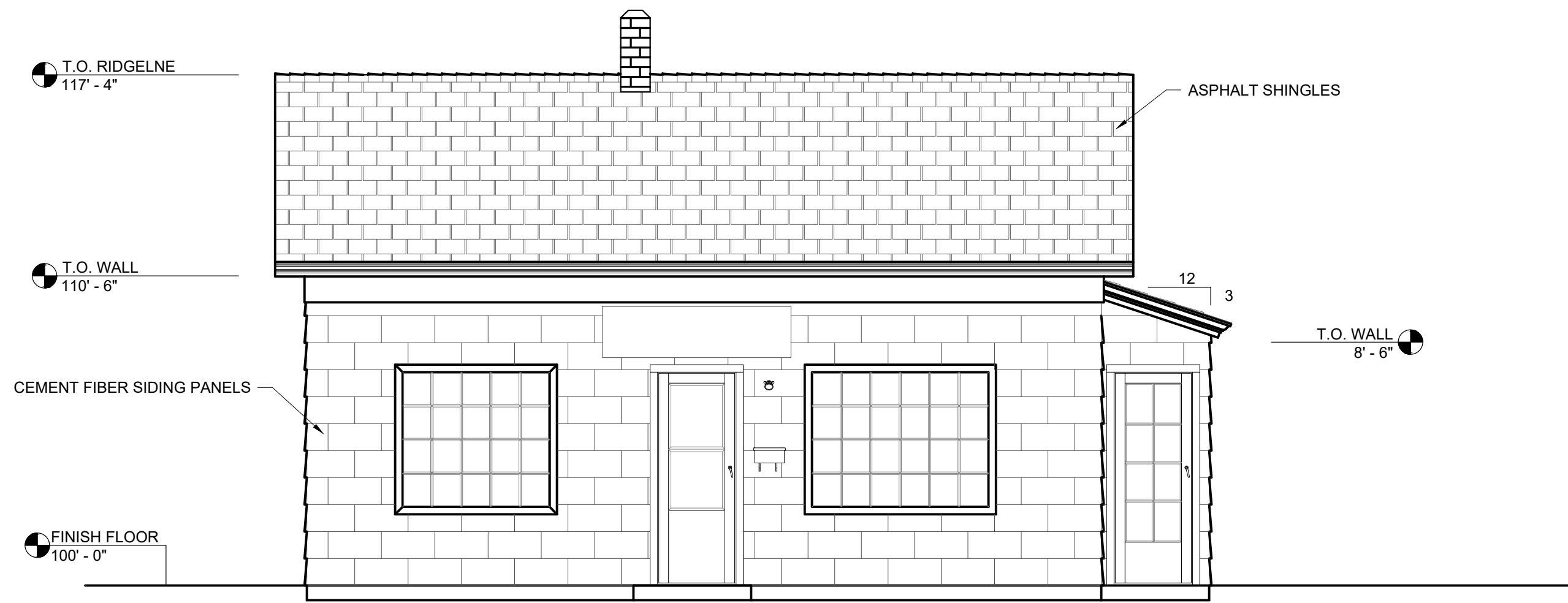
OFFICE WEST FRONT ELEVATION SCALE: 1/4"=1'-0"
