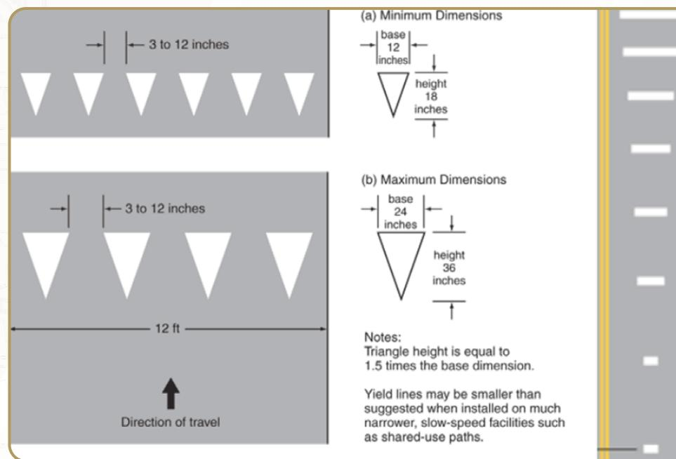
**FIGURE 34: Yield Lines and Advance Warning Markings (Source: MUTCD)**
