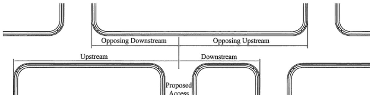
Figure 1: Measurements for minimum access spacing standards
