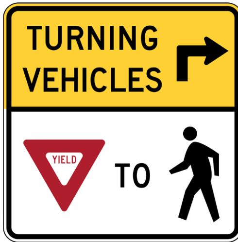
**FIGURE 37: R10-15 (L/R) Turning Vehicles Yield to Peds (Either Direction, Source: MUTCD)**
