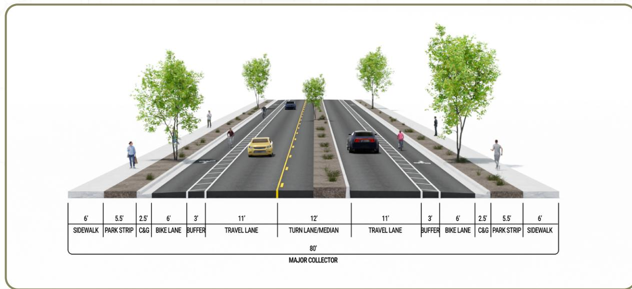
**FIGURE 7:** Major Collector Cross Section
