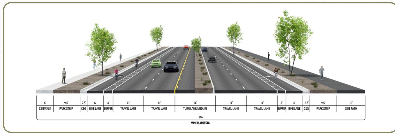
**FIGURE 6:** Minor Arterial Cross Section
