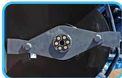
Two double-sided blades on a 5/8" thick blade carrier
