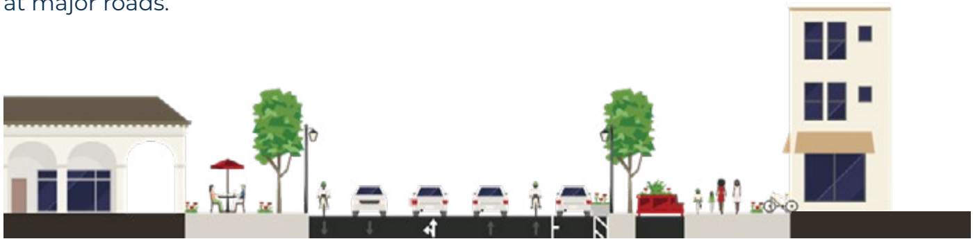
Figure 6. Within Mixed-Use Nodes Street Section
