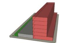
Recommended: Removal of unit minimum and unit/acre cap allows for more conventional, cost-effective urban construction
