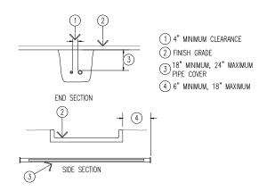
SLEEVES TO BE 2X PIPE SIZE WITHIN. JOINTS TO BE WATERTIGHT. MECHANICALLY ALL WIRE SLEEVING SHALL BE GRAY S/40 ELECTRICAL CONDUIT. NO EXCEPTIONS.
