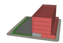
Recommended: Increased height limits, lower parking standards and removal of setbacks produces cost-effective 4-over-1 mixed-use building with tuck-under parking.
