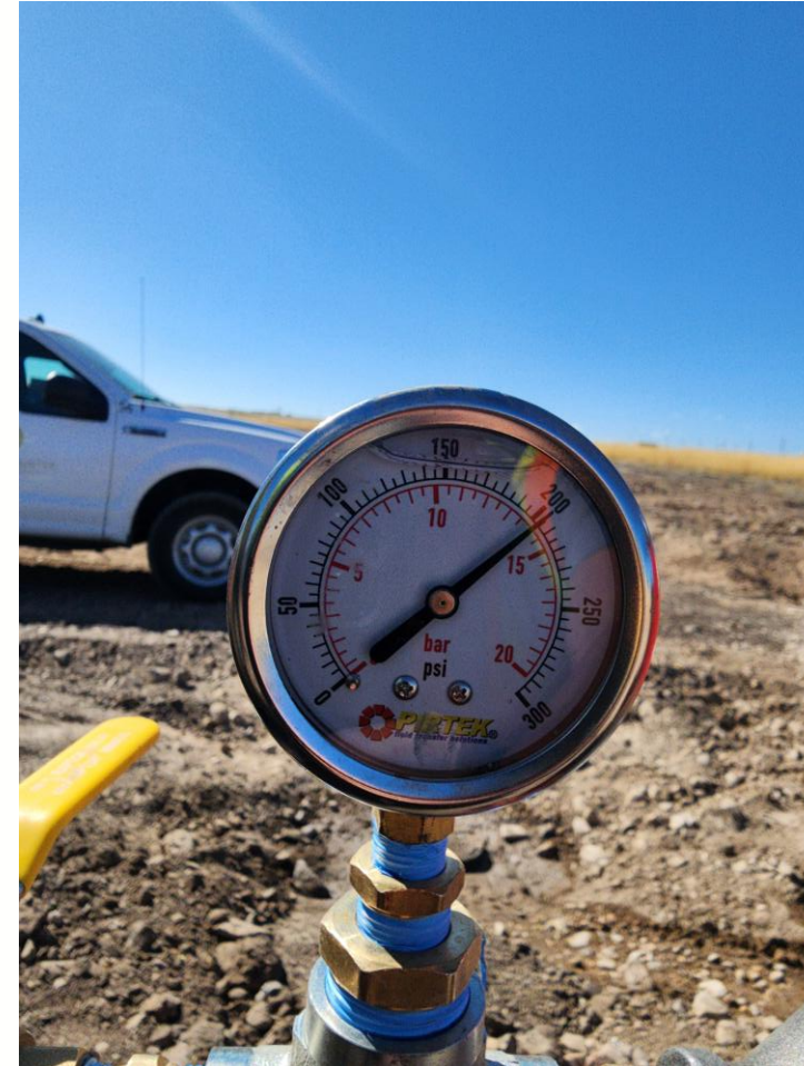
Pressure gauges for water main testing
