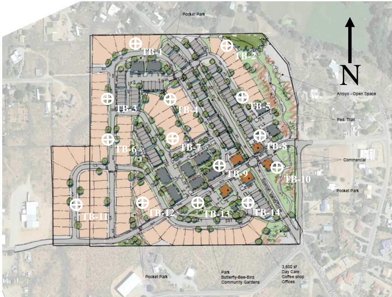
Figure 3.4: Approximate Test Boring Locations Relative to Preliminary Project Layout
