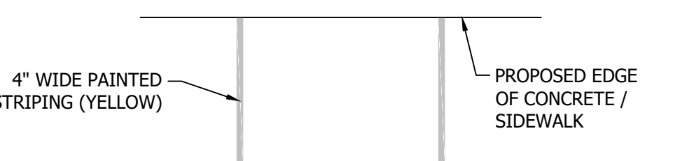
3 Typical Parking Space Scale: NTS
