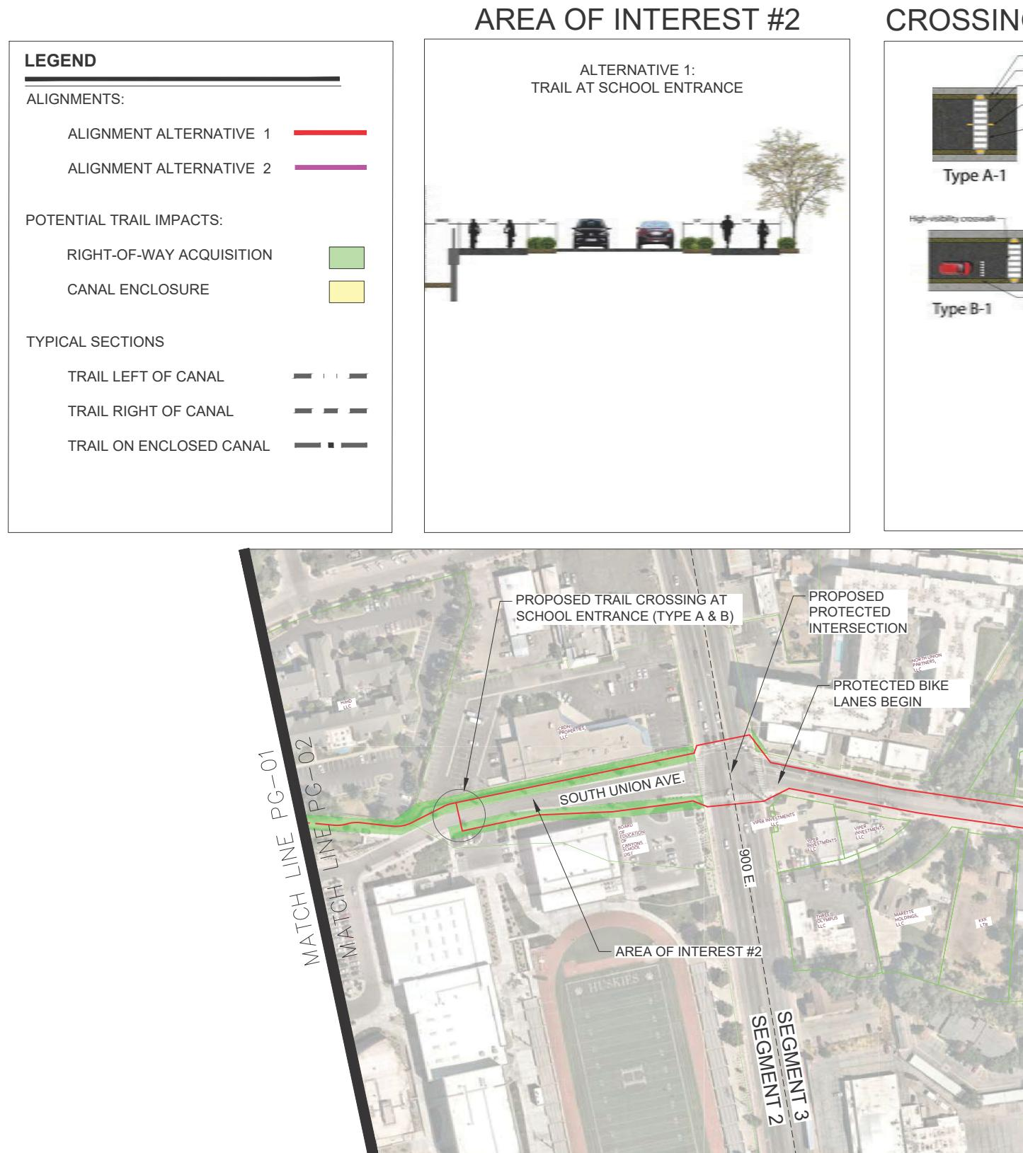
Figure 23: Proposed alignment along the East Jordan Canal, sheet 2.
