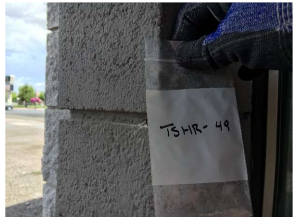
Photo #70 HA70: Mortar, not asbestos containing
