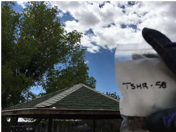
Photo #73 HA73: Black asphalt roof shingles with gray/green pebbles, not asbestos containing
