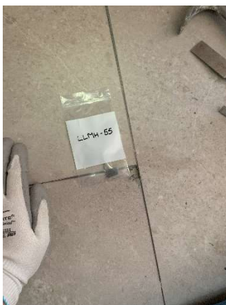
Photo #17 HA16: Gray 12"x24" floor tile and mastic, not asbestos containing
