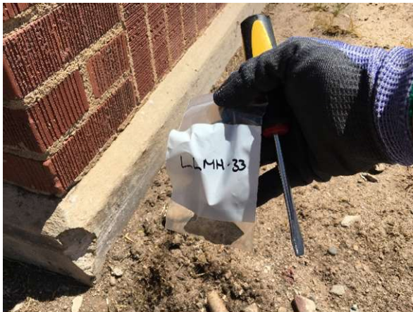
Photo #9 HA8: Concrete, not asbestos containing
