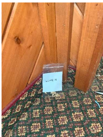
Photo #35 HA34: Yellow/black carpet mastic, asbestos containing
