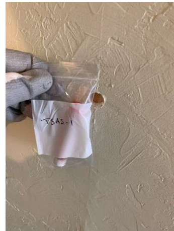
Photo #44 HA44: Gypsum board wall system, not asbestos containing
