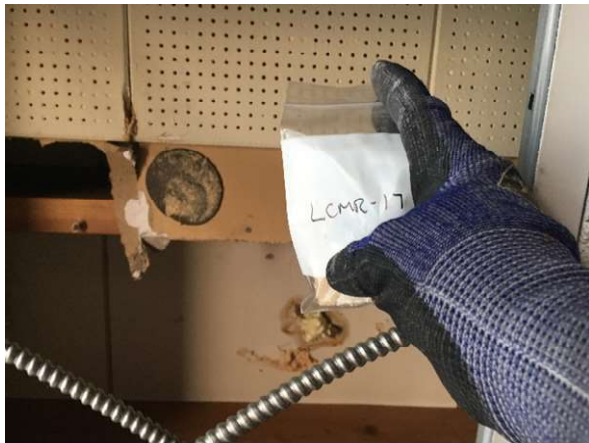
Photo #39 HA38: 1'x1' ceiling tile with hole punches and brown adhesive, not asbestos containing
