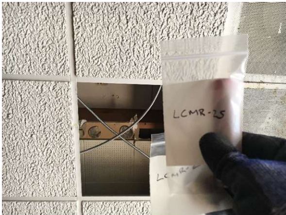
Photo #43 HA43: Tan fiber board ceiling panel, not asbestos containing
