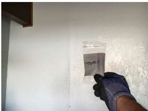
Photo #59 HA59: Gypsum board wall system, not asbestos containing
