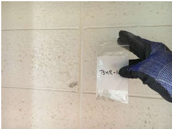
Photo #61 HA61: Interior paint on block, not asbestos containing
