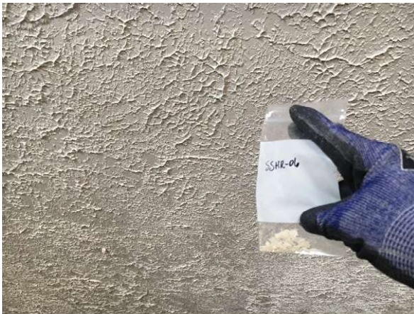
Photo #51 HA51: White ceiling texture, not asbestos containing
