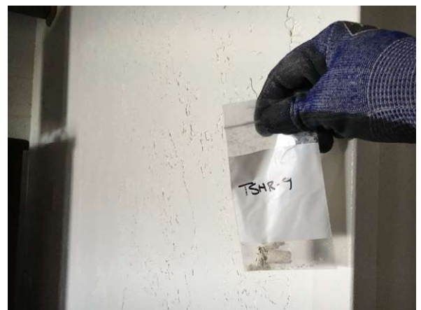
Photo #60 HA60: White "knockdown" wall texture, not asbestos containing
