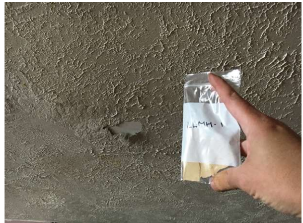
Photo #2 HA1: White rough ridge like ceiling texture, <1% asbestos by point count
