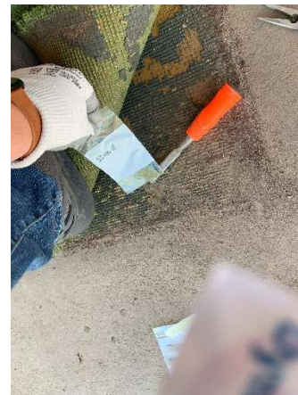
Photo #52 HA52: Yellow carpet mastic, not asbestos containing
