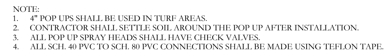
POP UP-SPRAY HEAD DETAIL NOT TO SCALE PKJ DESIGN GROUP
