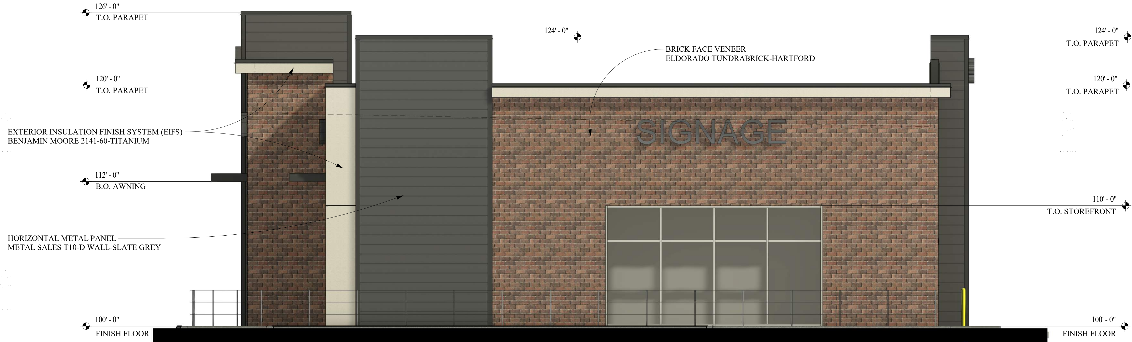
BLDG 'B' RIGHT ELEVATION - EAST 1/4" = 1'-0"
