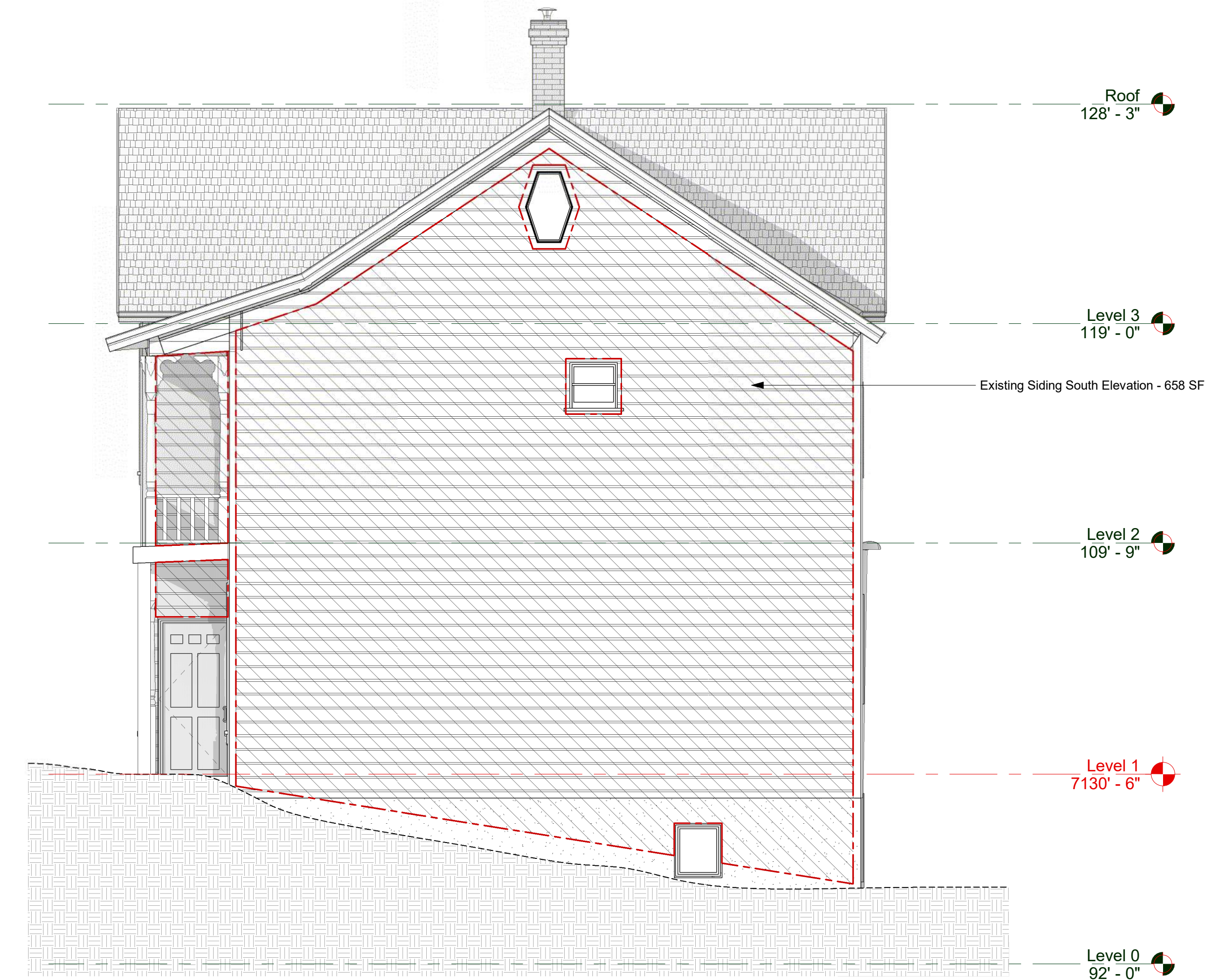
3 South Elevation - Siding 1/4" = 1'-0"
