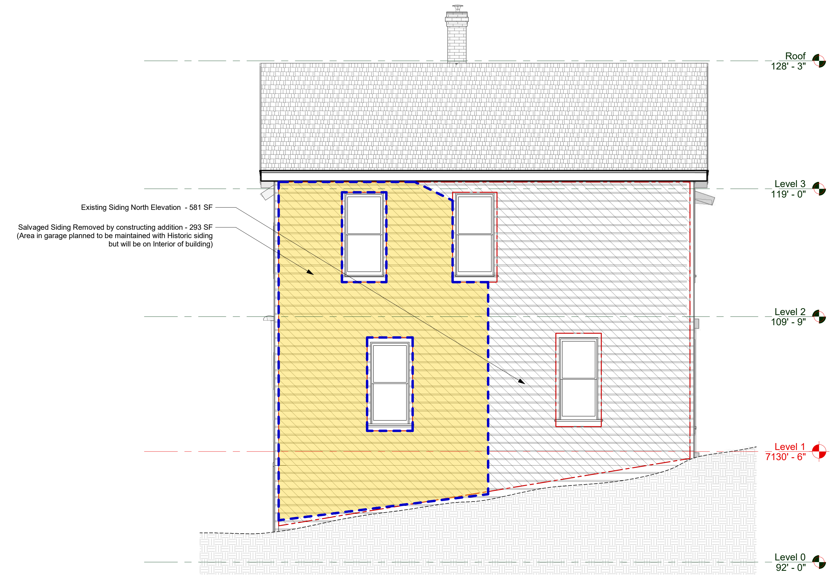
2 North Elevation - Siding 1/4" = 1'-0"
