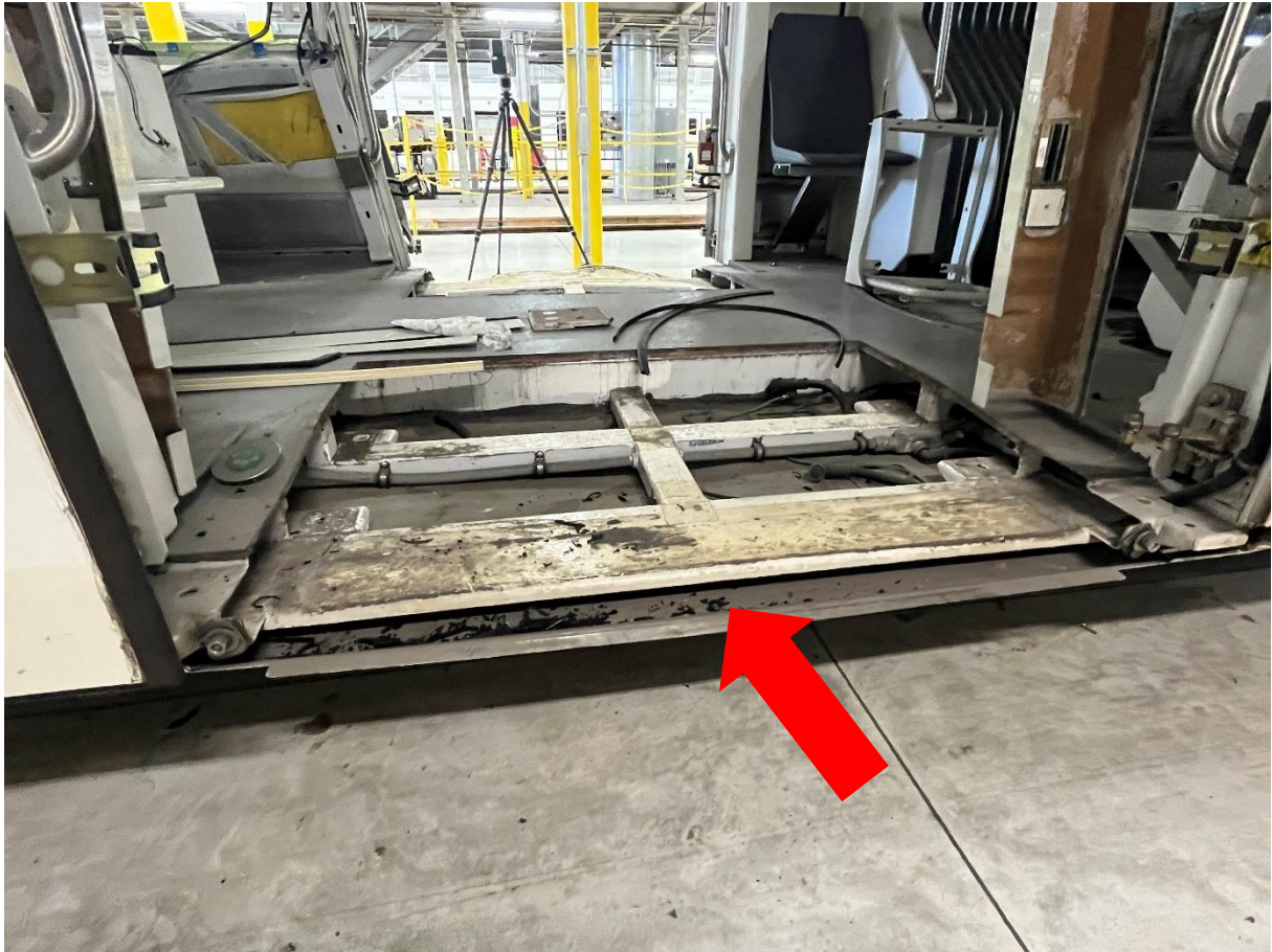
LH side "A" Car Damage to Door Threshold/Ramp A Slight Bending Observed Due to Impact on the Opposite Side
