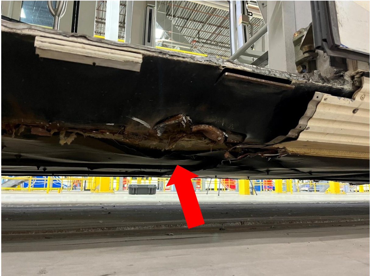
LH side “A” Car Damage to Door 11 Area Underside Bellypans
