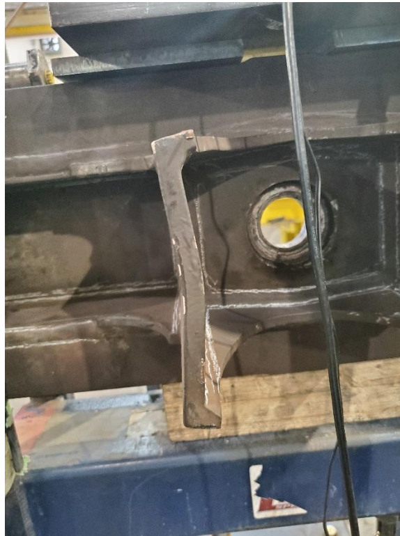
Figure 6: Damaged Bolster Lateral Bumper Stop.
