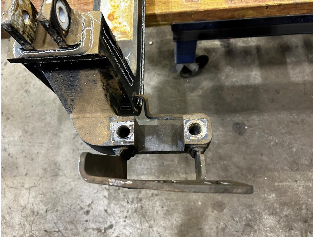
Figure 2: Affected headbeam console bracket.
