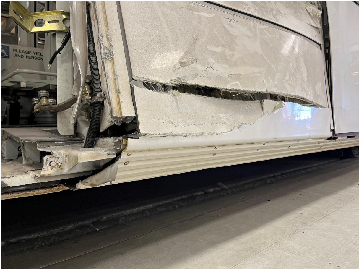
Impact Side View of Car body Between Doors 1-2
