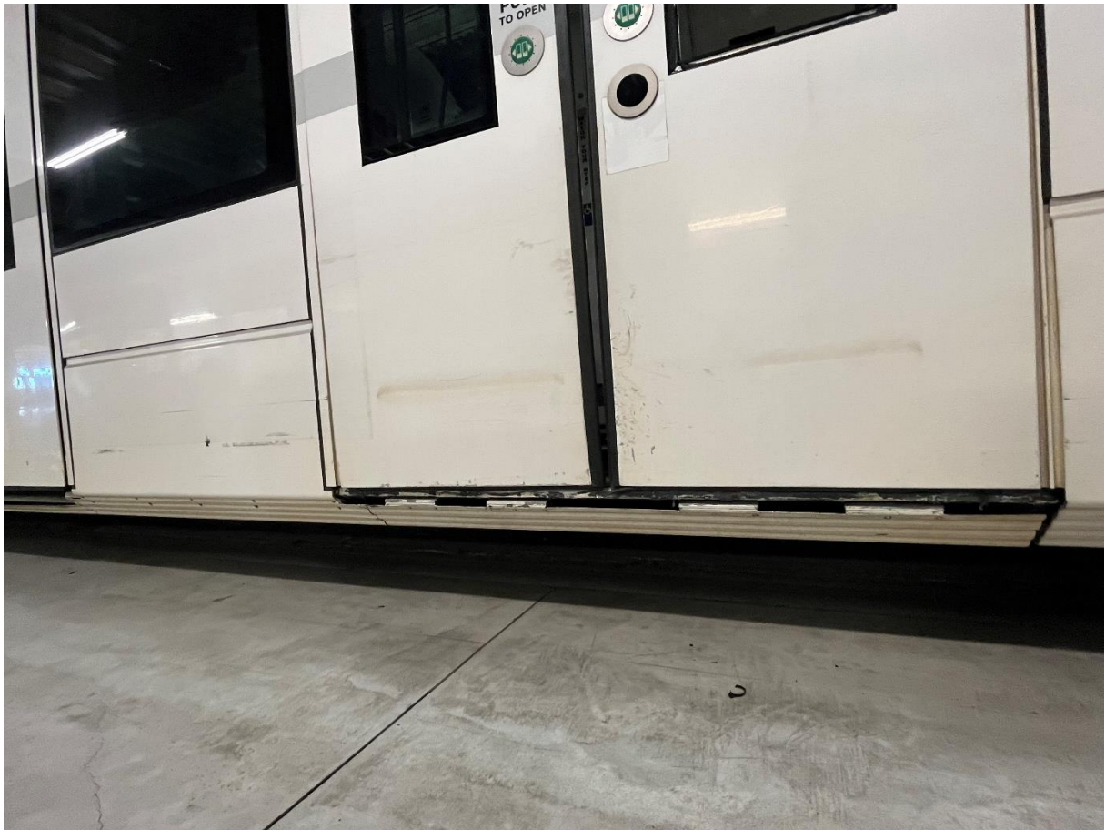
LH side "B" Car Minor Cosmetic Damage to Doors and Carshell
