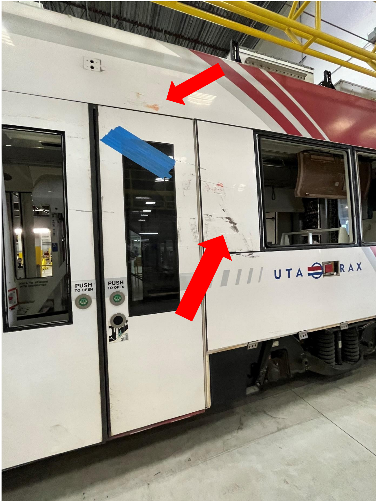
RH Side Door 1 and Carshell minor scrapes to “A” Car coatings – cosmetic damage
