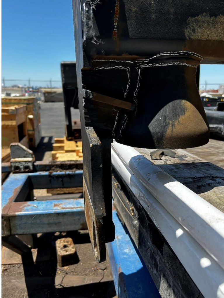
Figure 1: Track Clearer Bent Lifting Device Bracket
