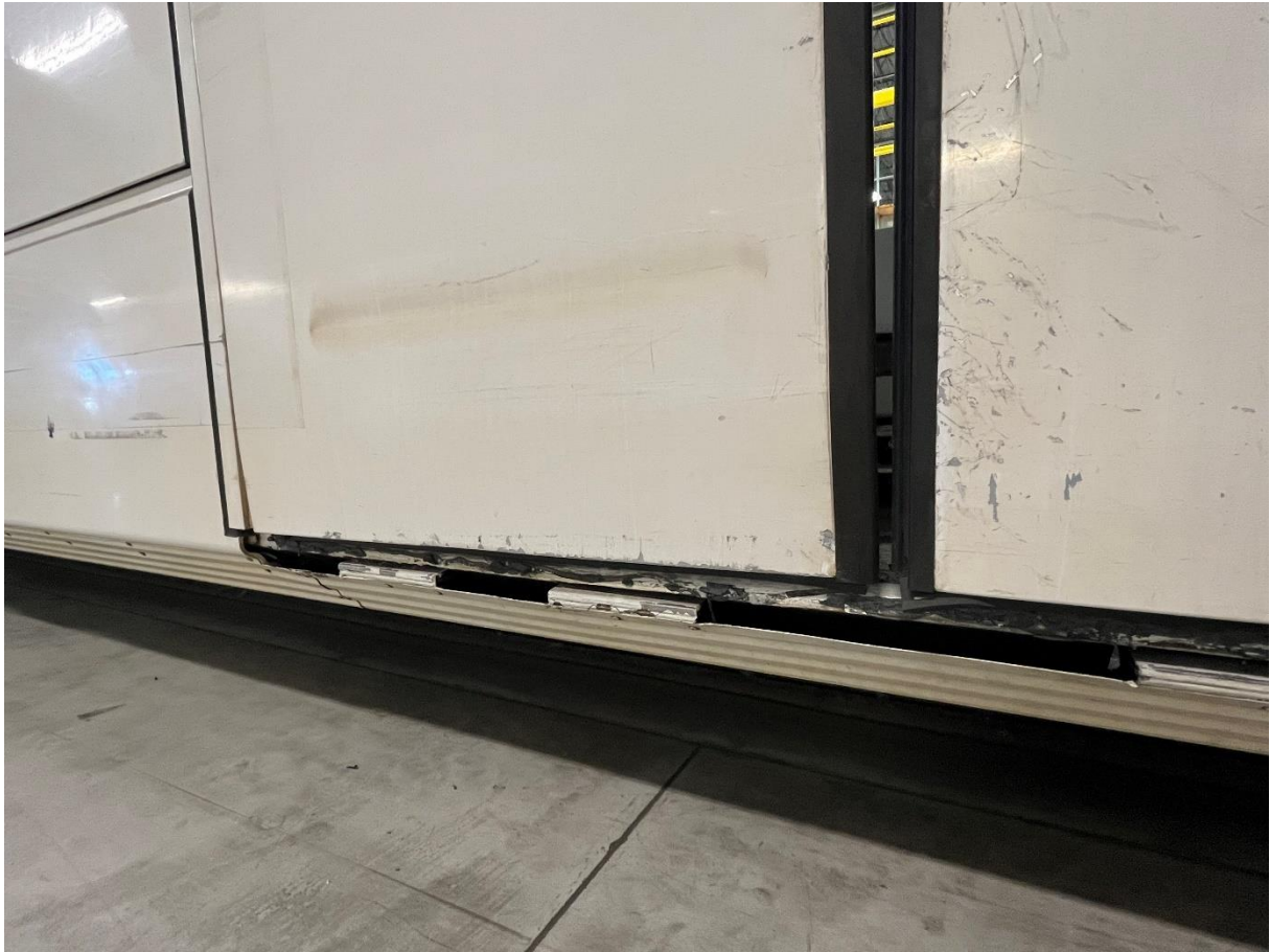
LH side “B” Car Damage to Doors and Carshell
