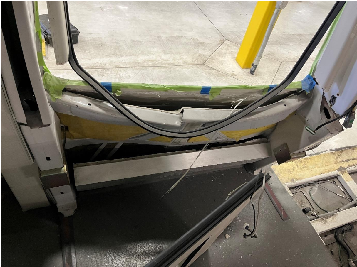
Window in Between Door 1 and 2 Interior View of Impact Damage
