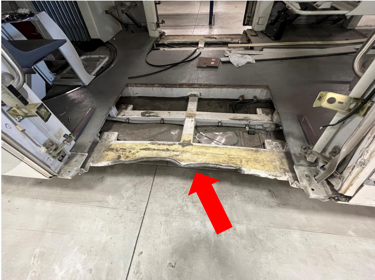
RH Side Door 2 threshold/Ramp Impact Area of "A" Car
