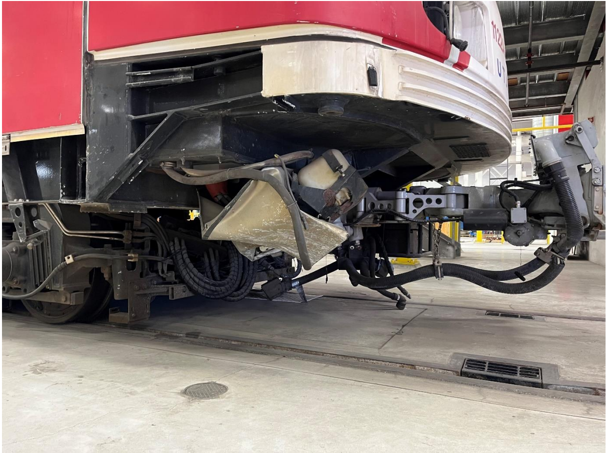
RH side 162 Box – damaged, including windshield washer reservoir
