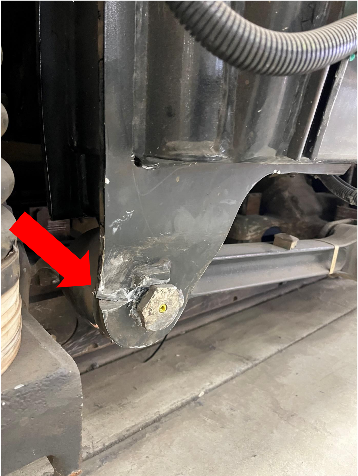
Truck traction rod RH bracket eye has a large crack/torn metal visible where the attachment bolt installs through the rod eye.
