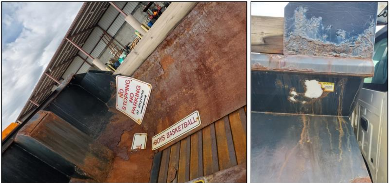
The Public Works Department has patched the holes in the sander bed using street signs to keep it operational.
