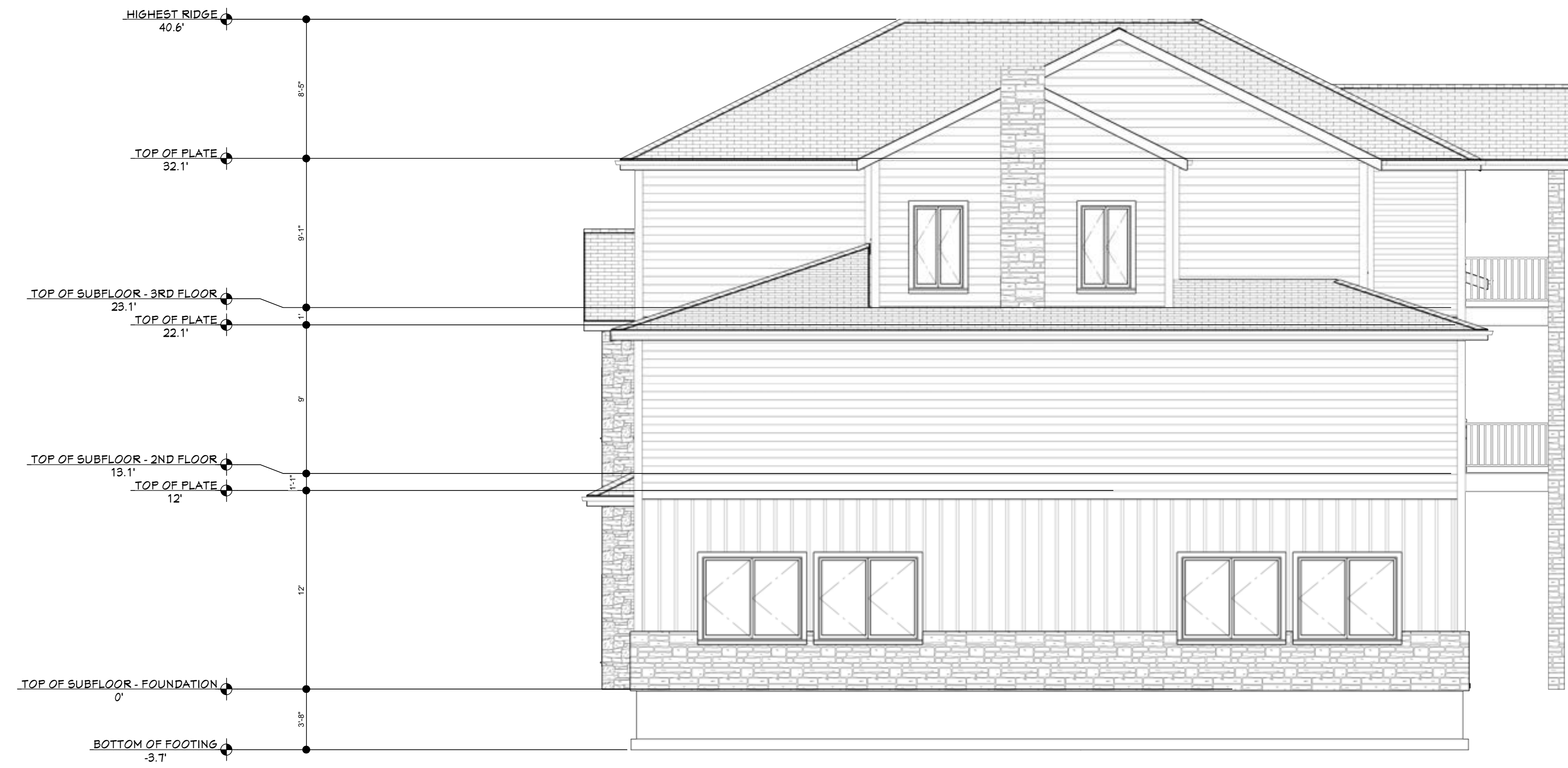
RIGHT ELEVATION VIEW 3/16"=1'-0"
