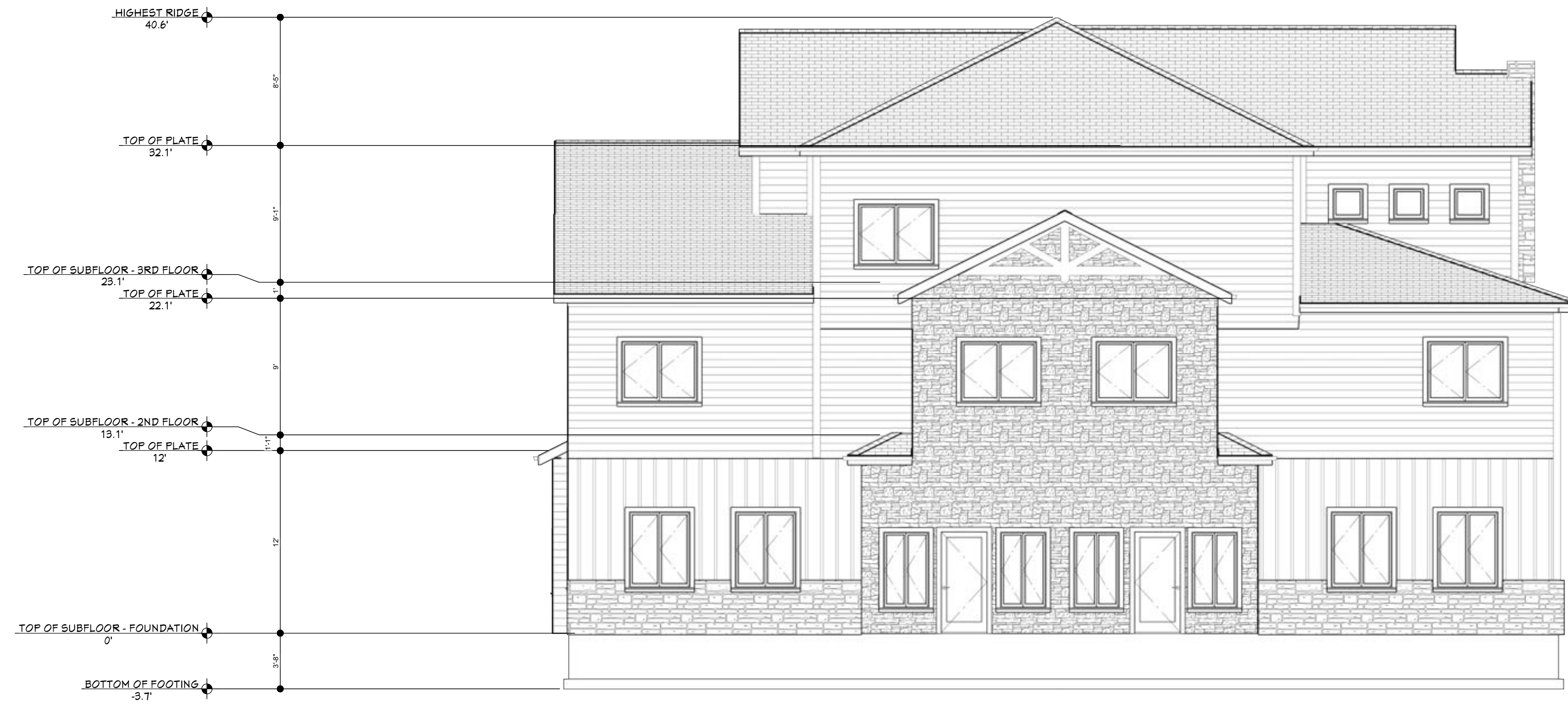
FRONT ELEVATION VIEW 3/16"=1'-0"
