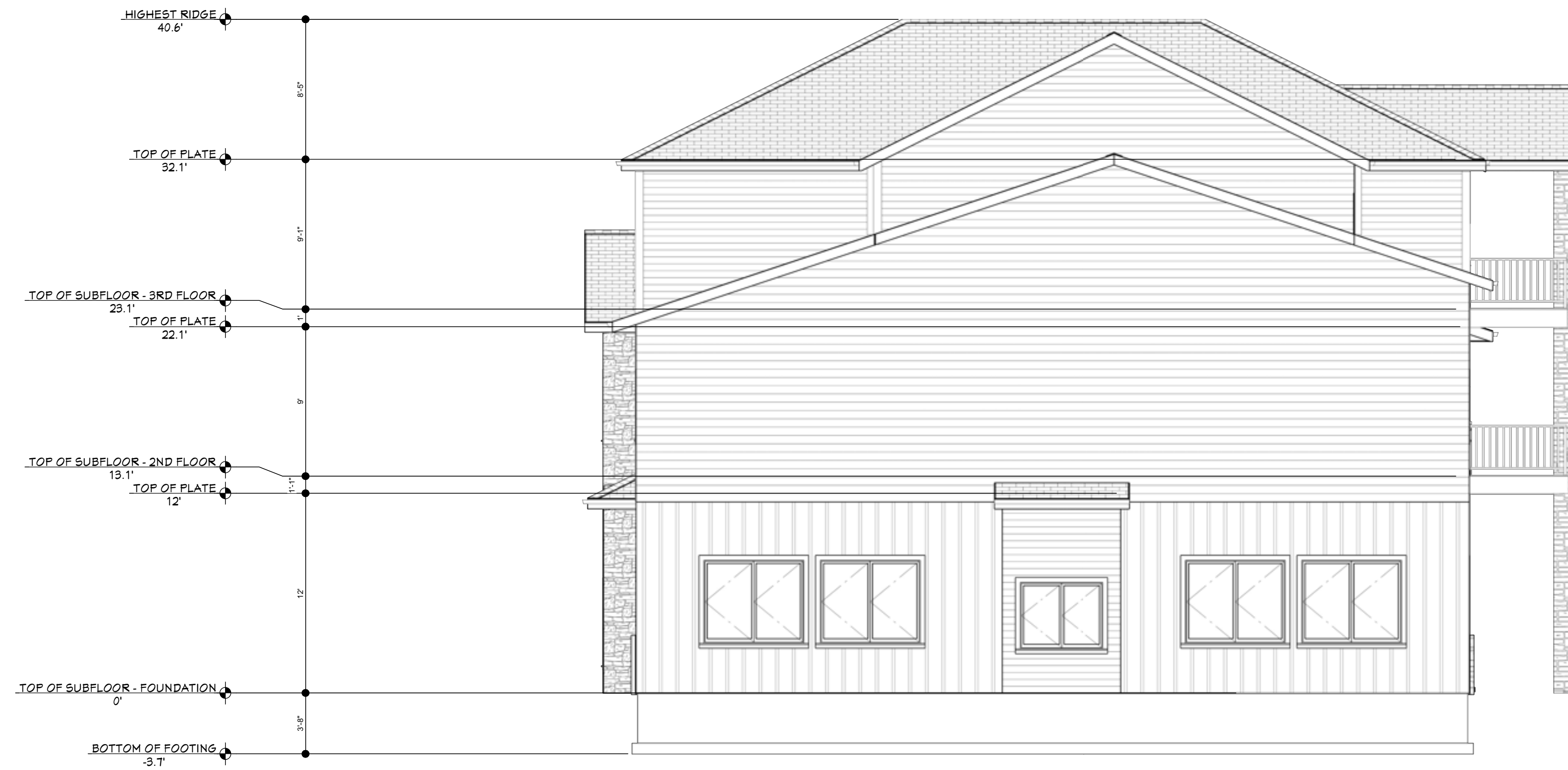
RIGHT ELEVATION VIEW 3/16"=1'-0"
