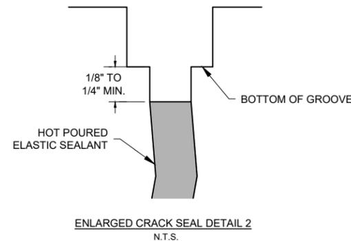
2 GROOVED RUNWAY CRACK SEAL DETAIL
