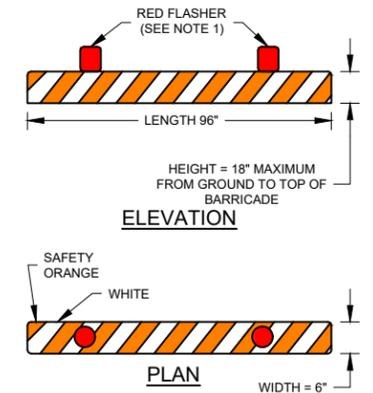
1. FLASHER BARRICADES WILL BE PROVIDED AND MAINTAINED BY THE CONTRACTOR AT ALL TIMES. CONTRACTOR SHALL ALSO PROVIDE SPARE BARRICADES, BATTERIES, AND LIGHT BULBS FOR MAINTENANCE DURING NIGHTTIME HOURS.
