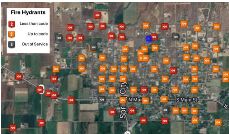
Slide 71 - Fire Hydrant Map of Spring City - Red is water pressure less than code, Orange is up to code, and Black is out of service - Internally tested
