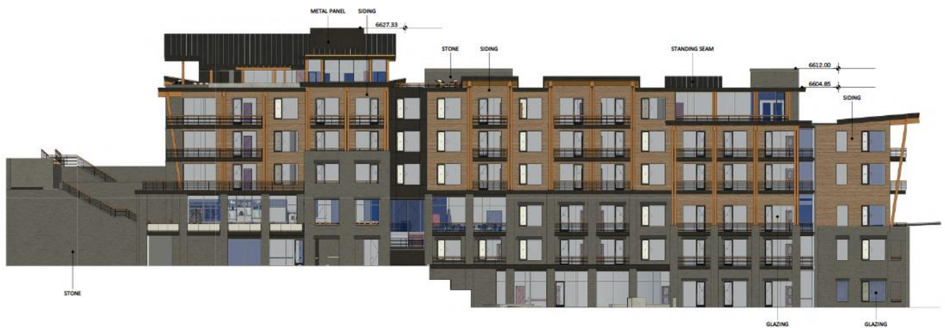
1 DR - SOUTH ELEVATION SCALE 1/16" = 1'-0"
