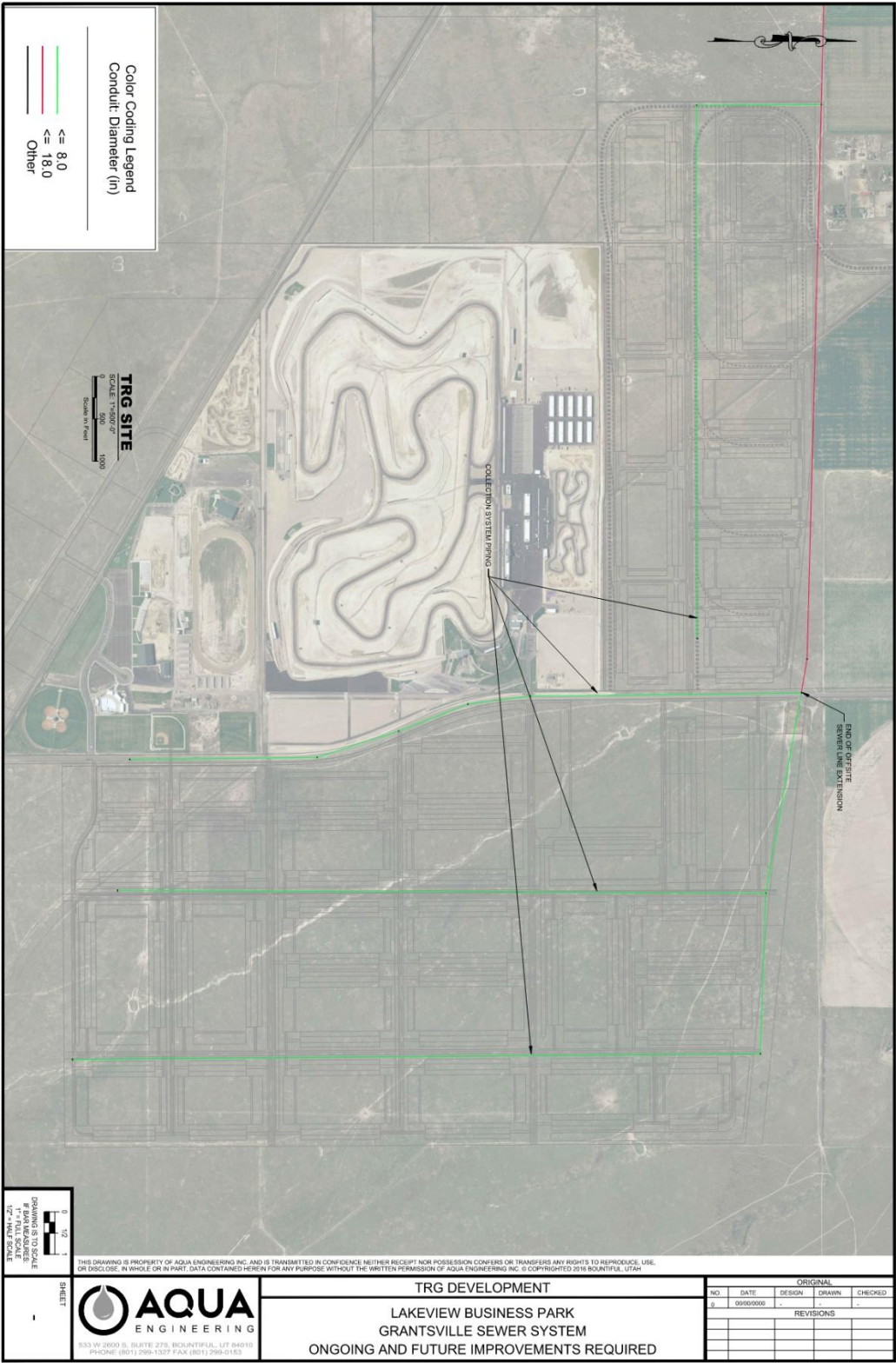
Figure 11: Ongoing and Future Sewer Improvements
