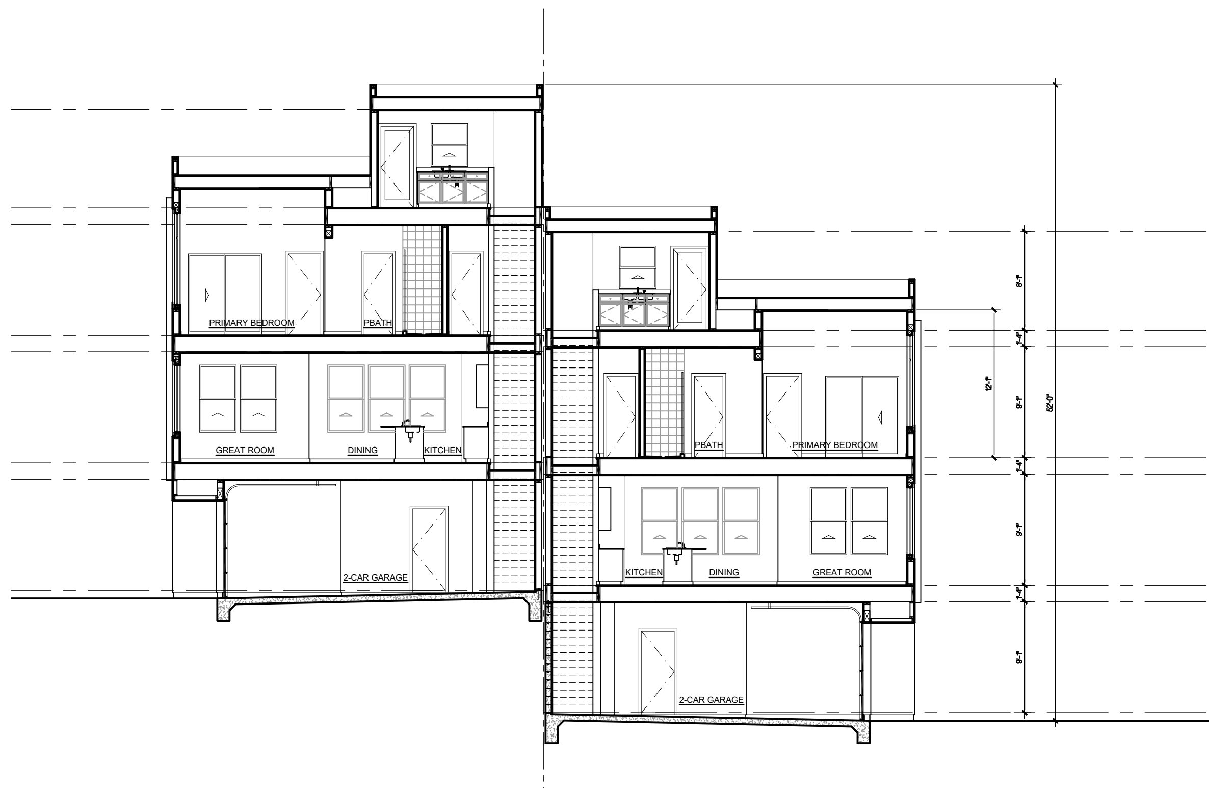
UPHILL/DOWNHILL BUILDING CROSS SECTION
