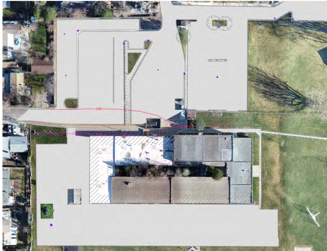
Partial Aerial Survey Showing Underground Utilities and Surface Conditions
