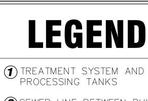
2 SEWER LINE BETWEEN BUILDING AND SEPTIC TANK SHALL HAVE 2% MIN SLOPE WITH ONE CLEANOUT MINIMUM. PIPE SHALL BE SOLID PIPE ON SOLID GROUND. ANY OVER EXCAVATION MUST BE BACKFILLED AND COMPACTED
