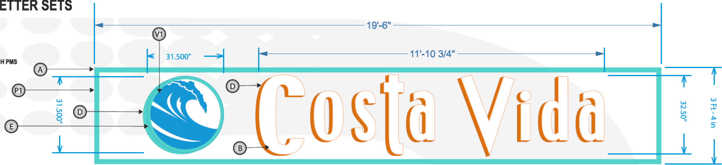
S1 INTERNALLY ILLUMINATED CHANNEL LETTERS - WEST ELEVATION Scale: 1/2" = 1'-0" (11"x17" Page Size)
