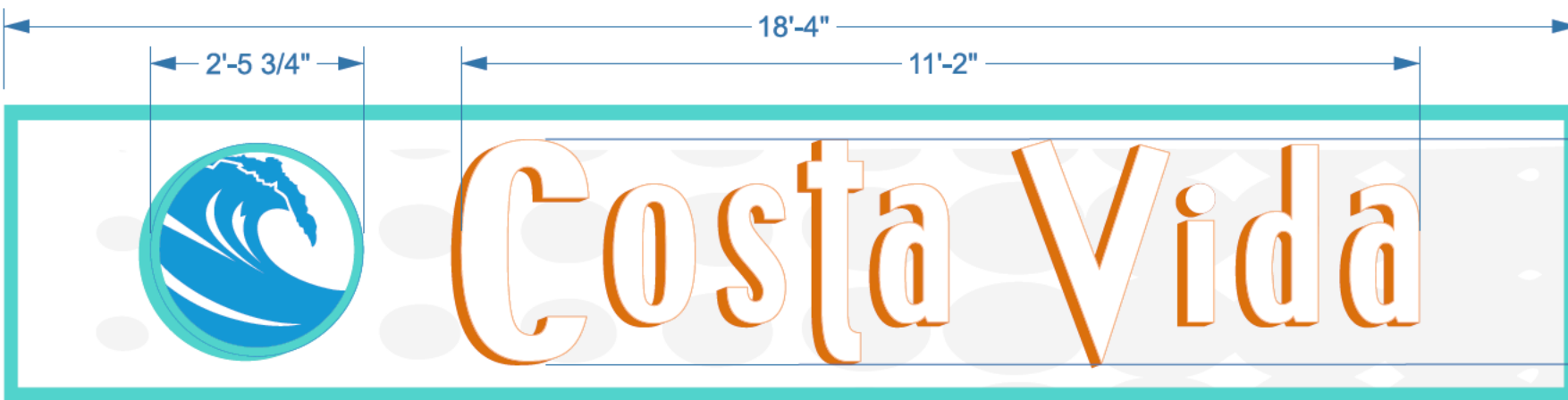
S1 INTERNALLY ILLUMINATED CHANNEL LETTERS - WEST ELEVATION Scale: 1/2" = 1'-0" (11"x17" Page Size)
