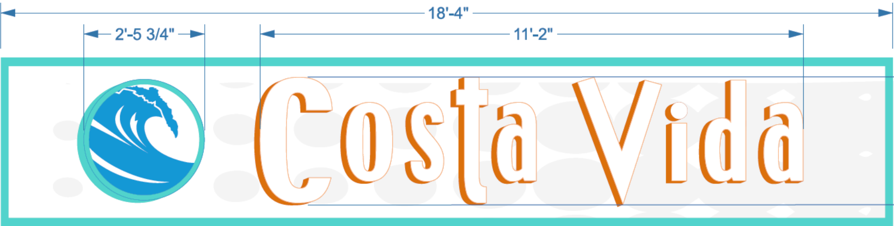
S1 INTERNALLY ILLUMINATED CHANNEL LETTERS - WEST ELEVATION Scale: 1/2" = 1'-0" (11"x17" Page Size)
