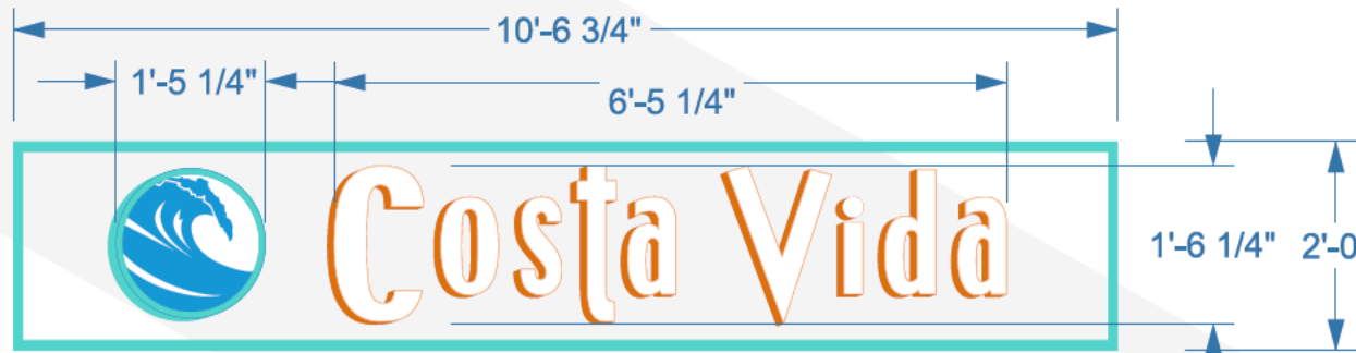
S3 INTERNALLY ILLUMINATED CHANNEL LETTERS - EAST ELEVATION Scale: 1/2" = 1'-0" (11"x17" Page Size)
