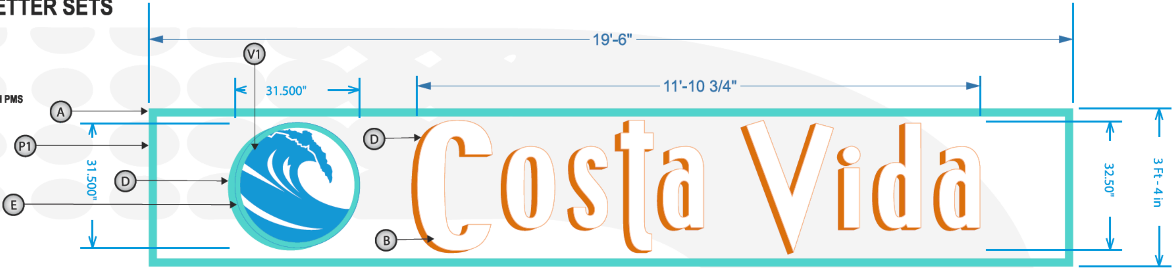
S1 INTERNALLY ILLUMINATED CHANNEL LETTERS - WEST ELEVATION Scale: 1/2" = 1'-0" (11"x17" Page Size)
