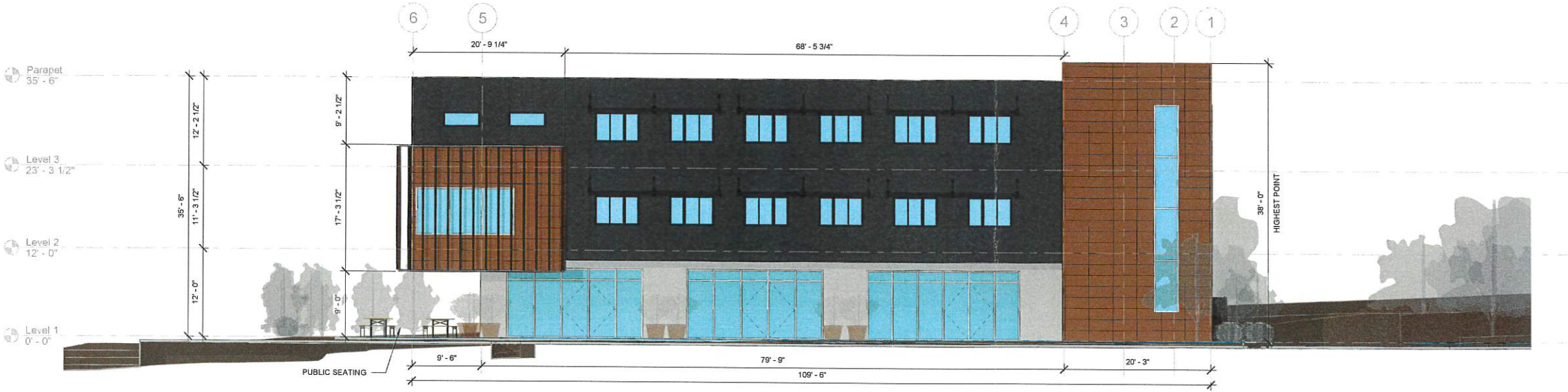
2 WEST ELEVATION - BUILDING FRONT, FACES LOT PARKING 1/8" = 1'-0"
