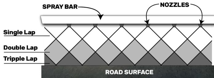
9. Spray nozzles must be evenly spaced and angled as shown:
