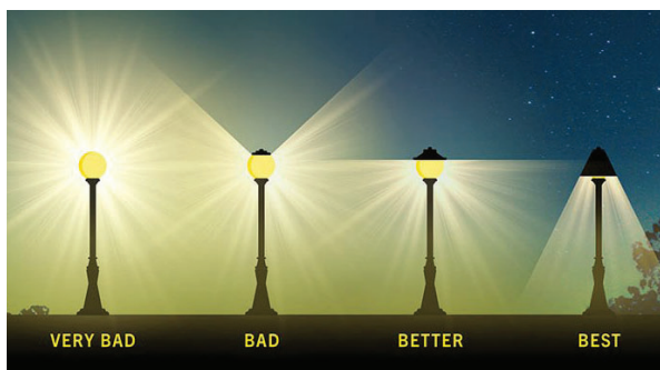
This graphic demonstrates how cut off fixtures are used to reduce light pollution
