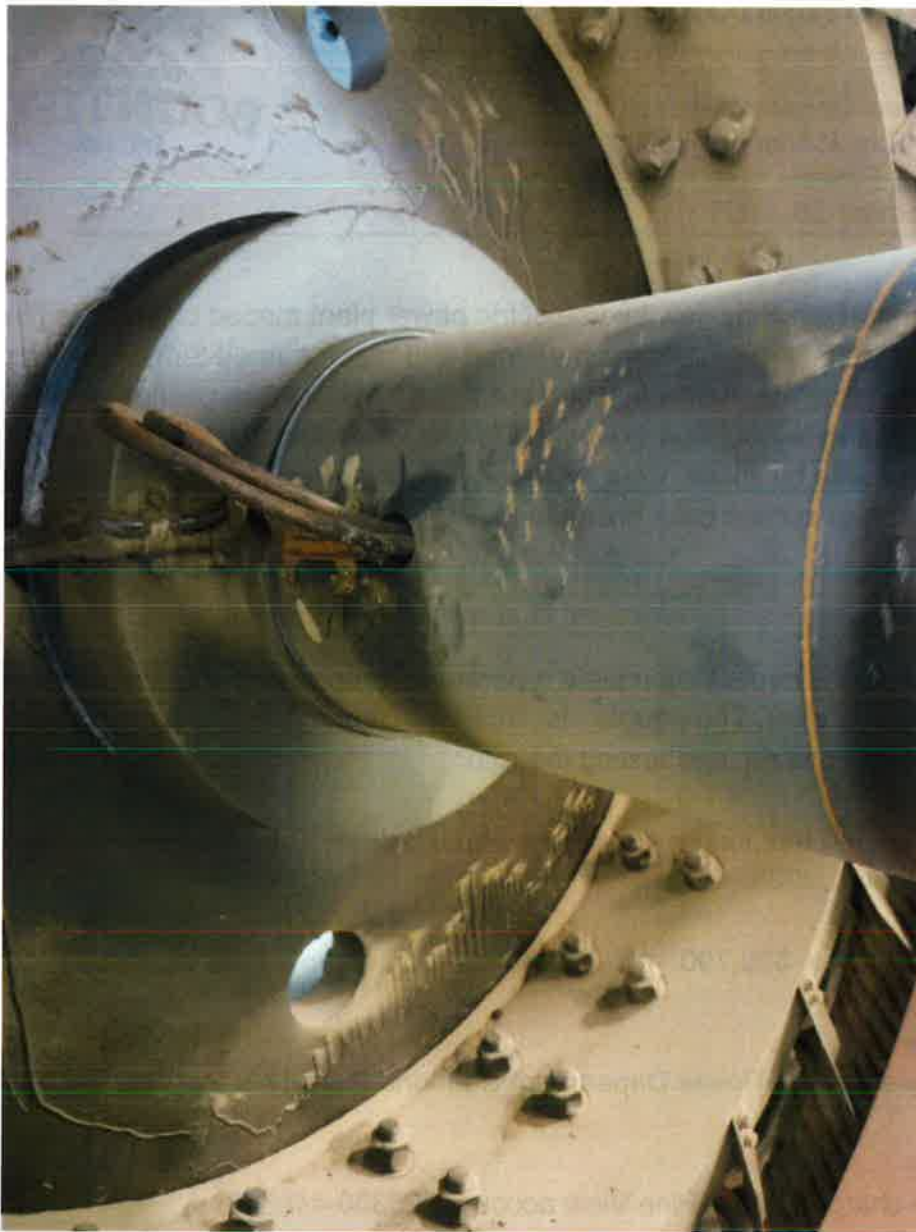
Shorted wire (the wire has been pulled out from the center of the rotor shaft)
