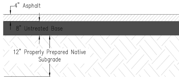
Pavement Section Typical
