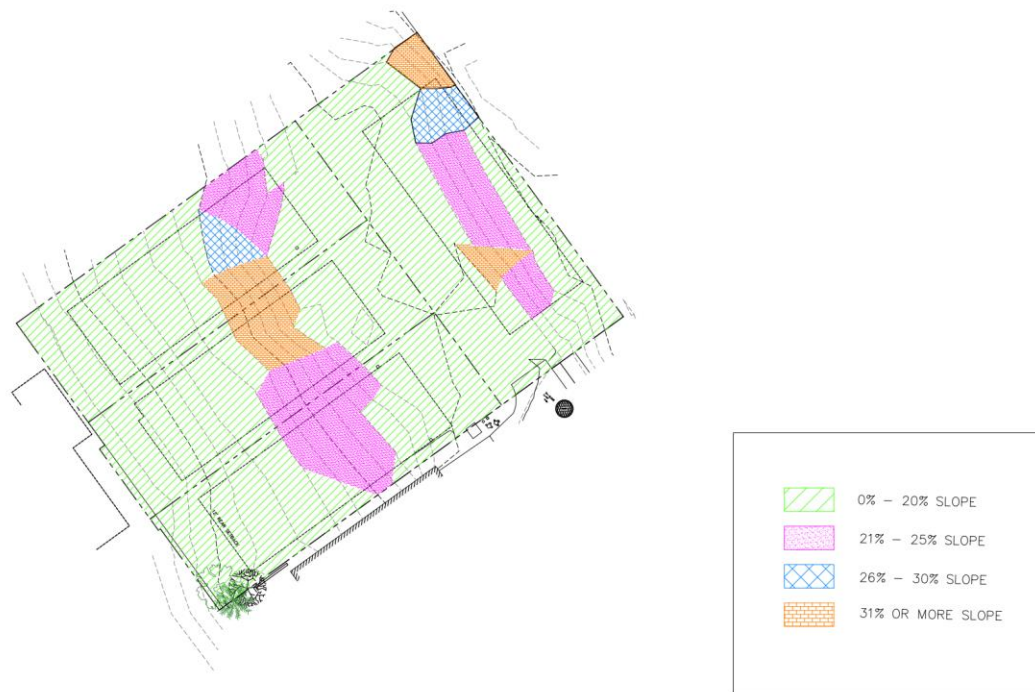
Figure 6: Slope Analysis Provided by Applicant (does not show up to date Building Pads)
