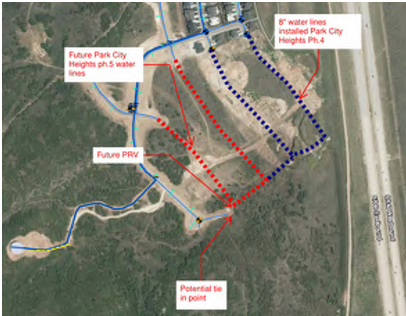
Illust. 171 - Conceptual Water Connection layout
