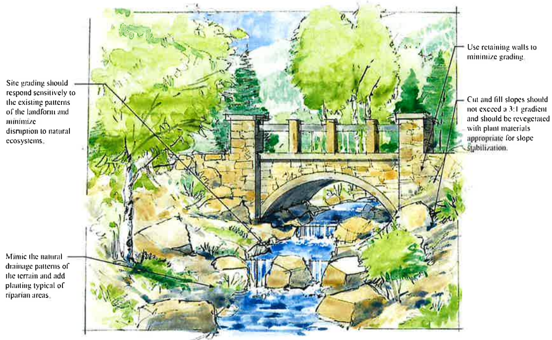
Figure 8: Grading and Drainage
