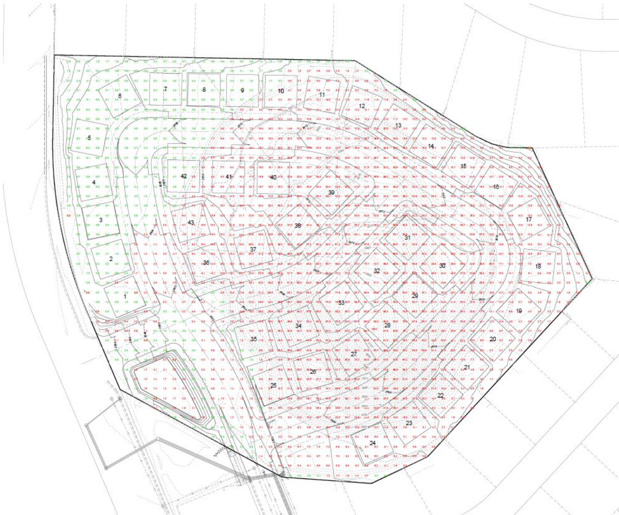
Figure 4, cut-fill map of the proposed grading, showing 42 lots, prepared by B&G.
