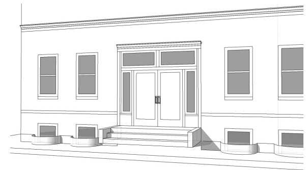
Figure 5.49 - Stoop entrance example, with visible basement
