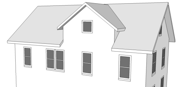
Figure 5.52 - Parallel ridge line with gable example
