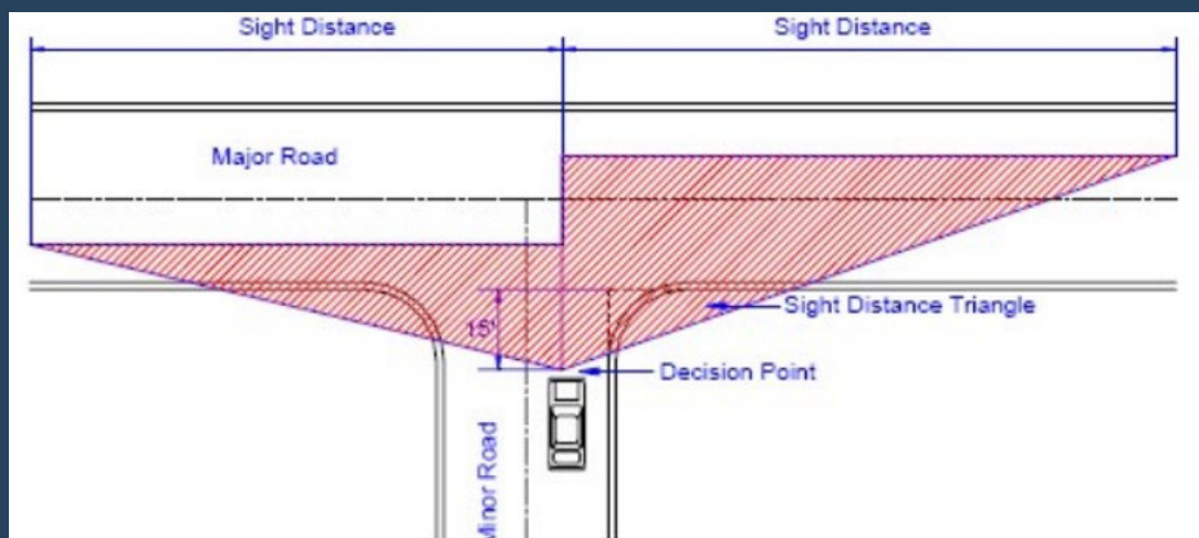
Figure 7: Sight Distance Triangle
