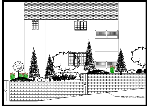
Proposed Retaining Wall
