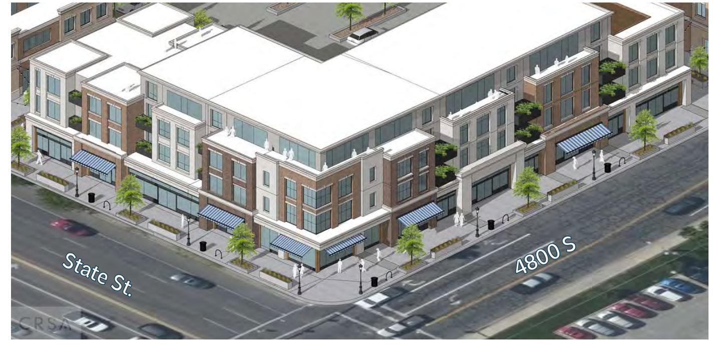
This rendering is an aerial view of the recommendations' largest building at the intersection of 4800 S and State St, featuring step-backs and patios on the fourth floor. Adding a stepback past the third floor is a key feature of the recommendation.
