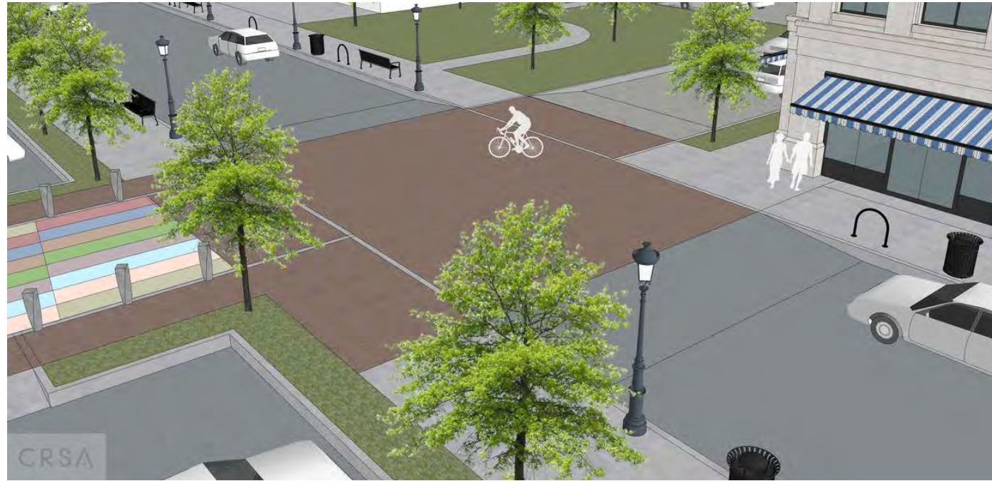
This rendering depicts the proposed improvements to the intersection of the alleyway and 5th Ave. Key improvements include a painted alleyway, bollards to protect pedestrians, added trees, and a speed table.
